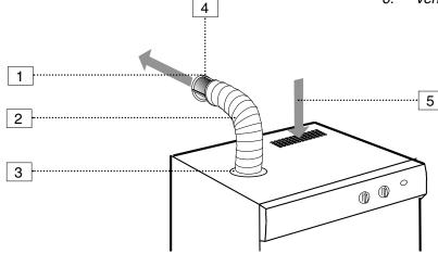
The drying cabinet is connected to the evacuation duct with a draft stabilizer
